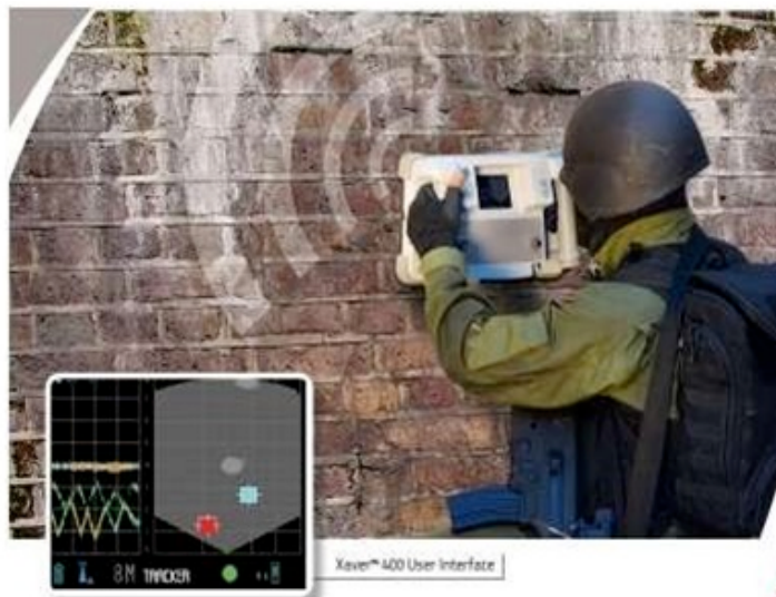
Figure 1. The compact translucent walls radar Source: Brochure XaverTM 400 www.camero-tech.com
